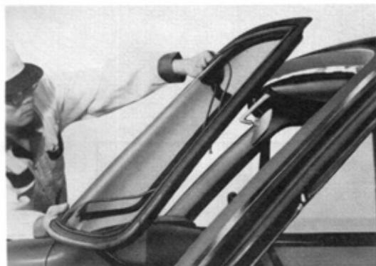
Fig.1-61 Glass Installation V0929
