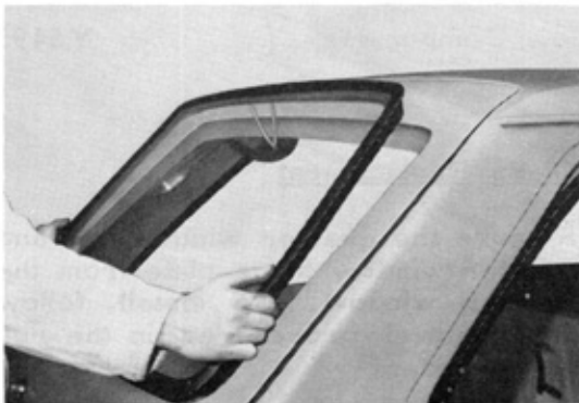
Fig.1-141 Glass Installation V3084
