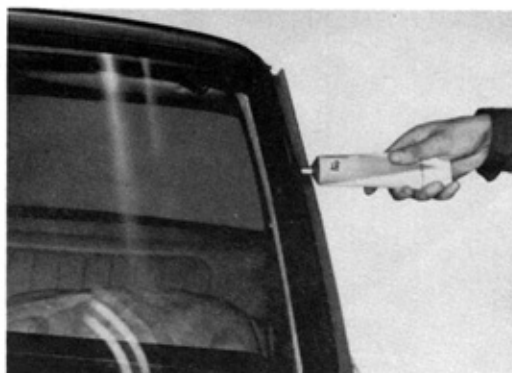
Fig.1-63 Applying Adhesive Cement V0931
